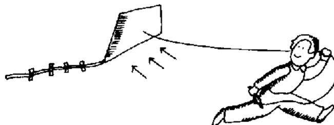
The front edges of the wings of a real aeroplane are usually tilted slightly upwards. As with a kite, the air pushes against the tilted underside of the wings, giving the plane lift. The greater the angle of the tilt the more wing surface the air pushes against. This results in a greater amount of lift. But if the angle of the tilt is too great, the air pushes against the larger wing surface presented and slows down the forward movement of the plane. This is called drag.
