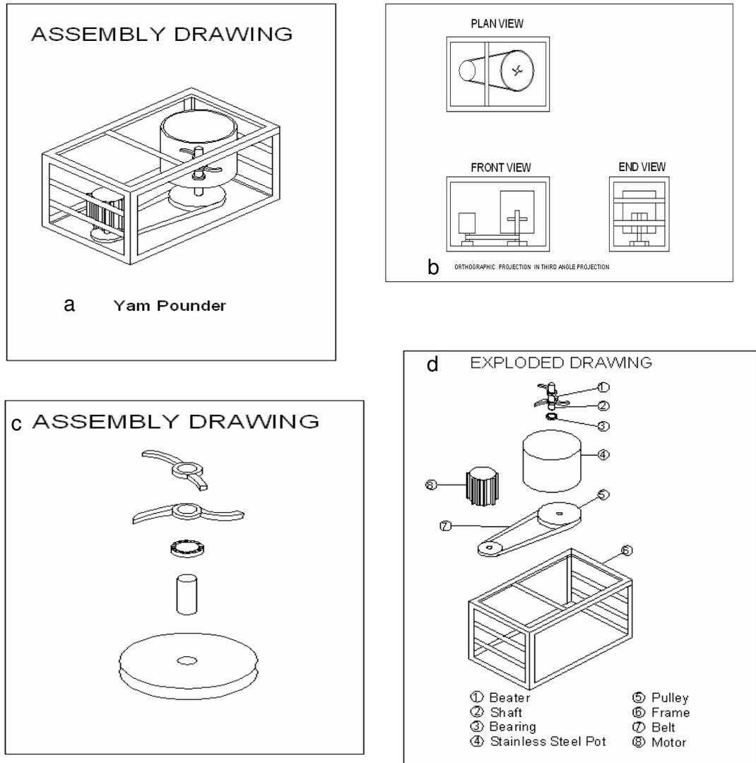
Fig. II: Component Elements of the Yam Pounding Machine
