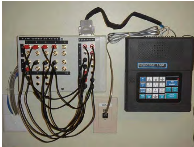
Fig. 1: Example of a small laboratory equipment alarm system based on the Sensaphone 1108 unit. Note the patch panel on the left, using RCA “phono” type connectors and short audio leads as patch cables.
