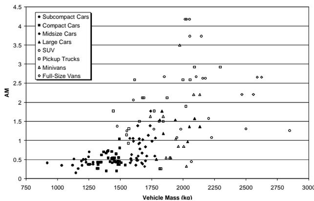
**Figure 8. Aggressivity as a function of Vehicle Mass.**
