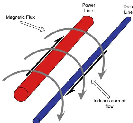
The solution to this particular problem involves moving data carrying devices and/or cabling away from the source of EMI/RFI, or to provide additional shielding for the data devices and/or their cabling to reduce, or nullify, the effects of the EMI/RFI.
