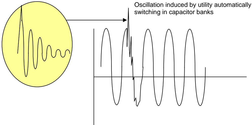
The most recognized problem associated with capacitor switching and its oscillatory transient is the tripping of adjustable speed drives (ASDs). The relatively slow transient causes a rise in the dc link voltage (the voltage that controls the activation of the ASD), which causes the drive to trip off-line with an indication of overvoltage.
