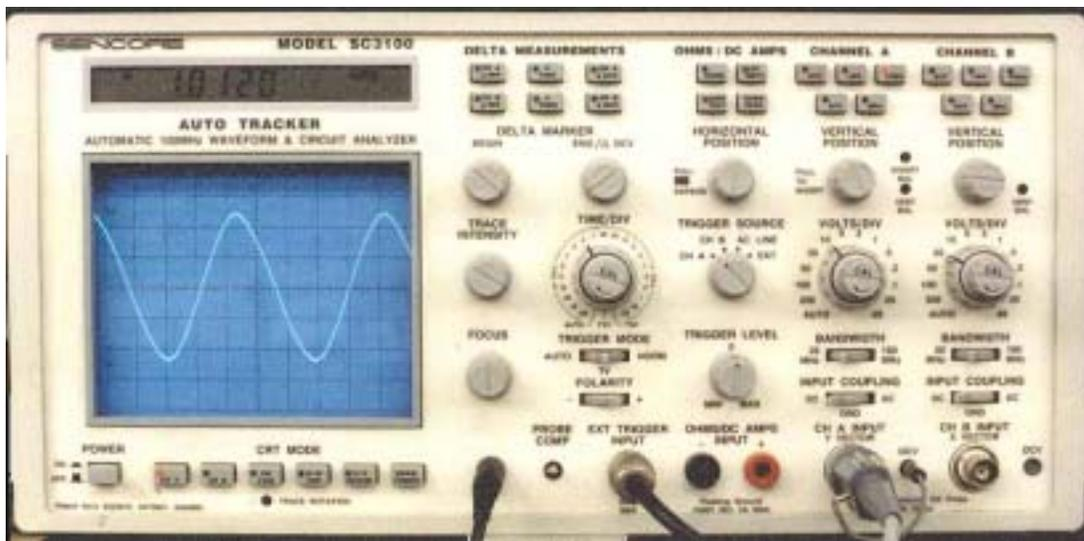
The sinusoidal wave shape shown above represents a voltage changing from a positive value to a negative value, 60 times per second. When this flowing wave shape changes size, shape, symmetry, frequency, or develops notches, impulses, ringing, or drops to zero (however briefly), there is a power disturbance. Simple drawings representative of changes in the above ideal sine wave shape will be shown throughout this paper for the seven categories of power quality disturbances that will be discussed.
