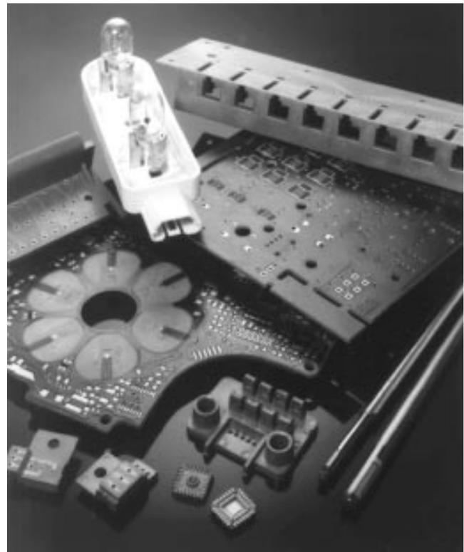
Fig. 2—Examples of commercially produced molded interconnect devices. (Courtesy of J. Rychwalski, Shipley Co.)
