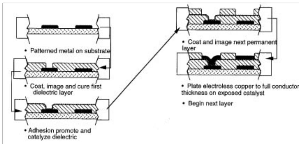
Fig. 4—Process flow for MCM-D on a conventional PWB. (Courtesy of P. Knudsen, Shipley Co.)
