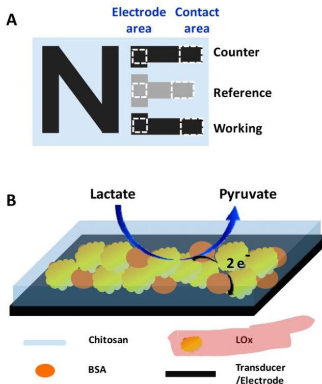
Figure 3 (A) Schematic of three-electrode "NE" tattoo biosensor for electrochemical epidermal monitoring of lactate. (B) Reagent layer of working electrode coated by biocompatible polymer (chitosan) [6].
