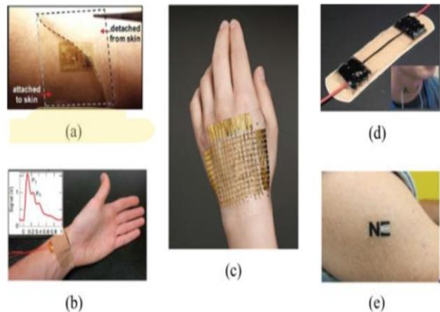
Figure 2. Flexible and stretchable wearable devices for healthcare applications developed by different groups [19].
