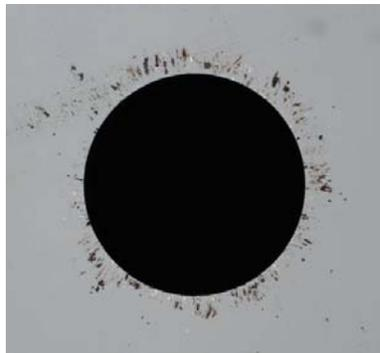
**Figure 11.** Natural diamond jewel orifice showing signs of wear, maintaining sharp leading edge.
