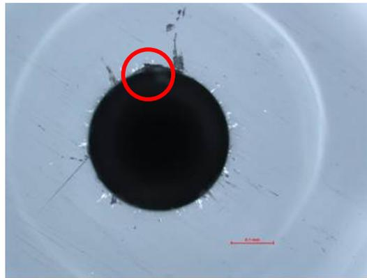
**Figure 9.** Sapphire orifice, sharp leading edge, chipping due to particulate material.
