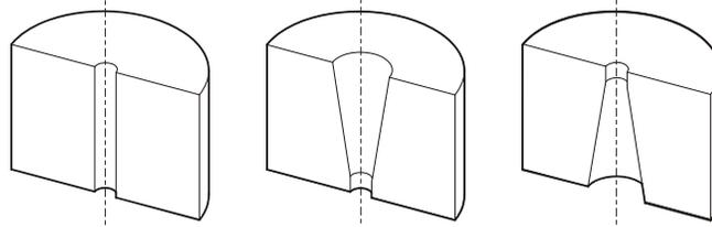
**Figure 7.** Orifice mount styles; cylindrical, cone-up, and cone-down [4, 5]
