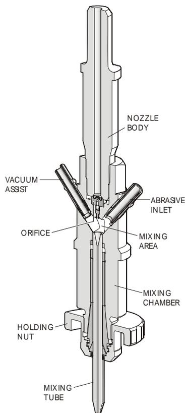
**Figure 2.** Diagram of high-performance abrasive waterjet cutting head
