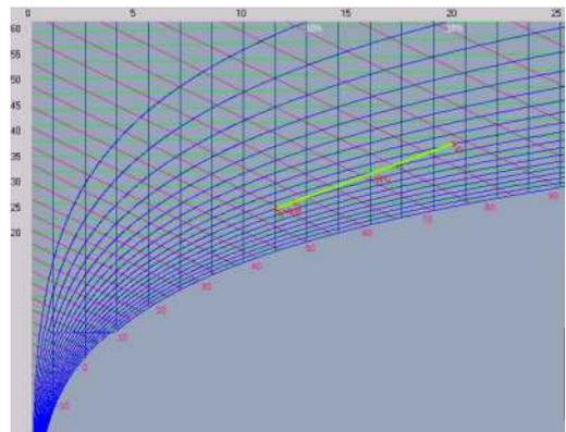
Fig 1 the psychrometric chart in the air treating process
