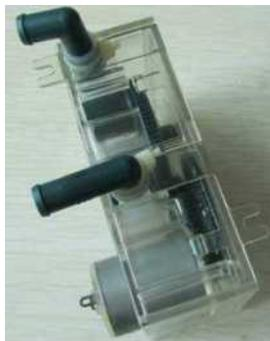
Figure 3 the diagram of peristaltic pump
