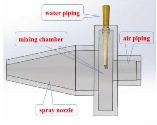
Figure 6 schematic diagram of spray nozzle
