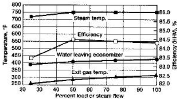
Fig. 4. Packaged boiler performance.
